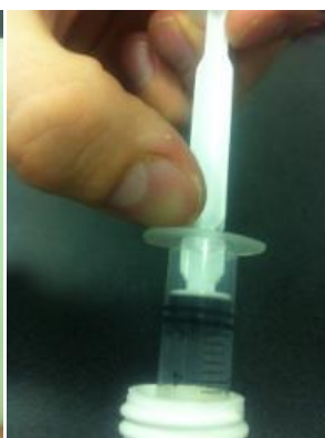
Figure 5. Withdraw the titrant from its bottle using a clean 5 mL syringe. If you are using the glass burette, use the syringe to fill it.
