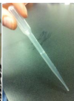
Figure 7. The transfer pipette. One full squeeze of the transfer pipette in either the Acid solution or Reactant should be approximately 2 mL.
