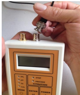
Figure 3. Be sure the pH electrode attachment is screwed into place on the BNC connector.
