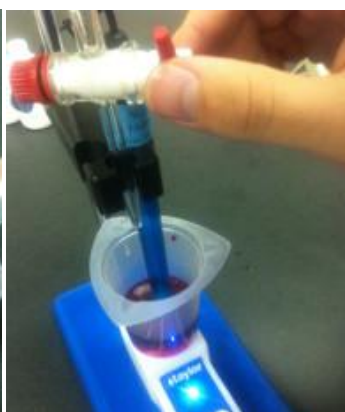
Figure 9. Automated stirring technique. Turn on the magnetic stirrer; add SO 2 Titrant by slowly opening the burette stopcock valve.
