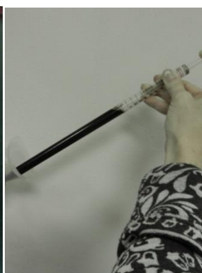
Figure 6. Dispense 25 mL of your wine into the titration beaker using the 25 mL sampling pipette. Make sure this is clean before putting the pipette into your wine container!
