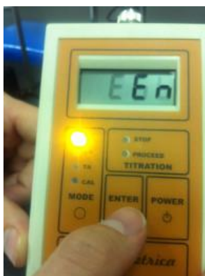
Figure 4. Once in SO 2 MODE the instrument should read 'Press Enter' Press ENTER to activate SO 2 MODE.
