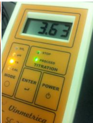
Figure 14. Make sure that the green "PROCEED" LED is lit. You should be reading a pH close to what you expect your wine is at. You are ready to titrate!
