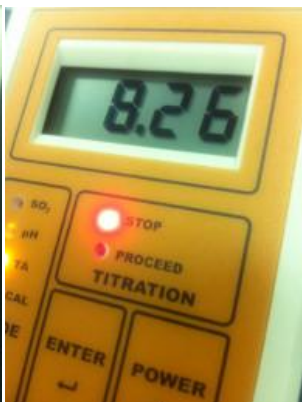
Figure 15. Once the pH arrives at or passes 8.20 you are done with the titration. The red "STOP" LED will be lit and the instrument will be beeping
