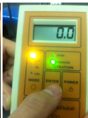
Figure 10. Make sure that the "PROCEED" LED is lit. You should be reading close to 0.0 when you first start. You are now ready to titrate!
