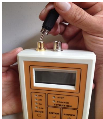
Figure 2. Attach the SO 2 electrode to the phono plug connector on the SC-300 by pushing it straight on. Avoid a twisting motion.
