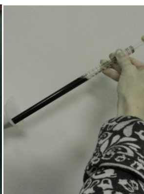
Figure 17. Dispense 25 mL of your wine into the titration beaker using the 25 mL sampling pipette. Make sure this is clean before putting the pipette into your wine container!
