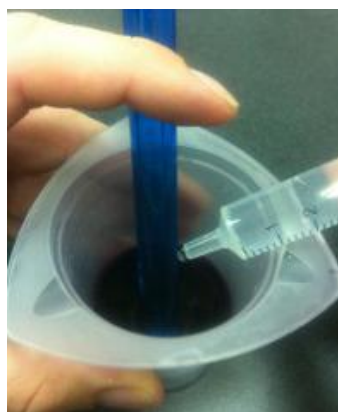
Figure 19. Manual stirring technique. Hold the electrode against the side of the titration beaker and swirl gently; add SO 2 Titrant with other hand.
