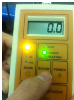
Figure 21. Make sure that the "PROCEED" LED is lit. You should be reading close to 0.0 when you first start. You are now ready to titrate!
