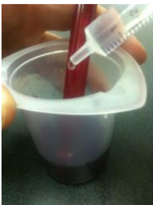
Figure 23. Manual stirring technique. Hold the electrode against the side of the titration beaker and swirl gently; add TA Titrant with other hand.
