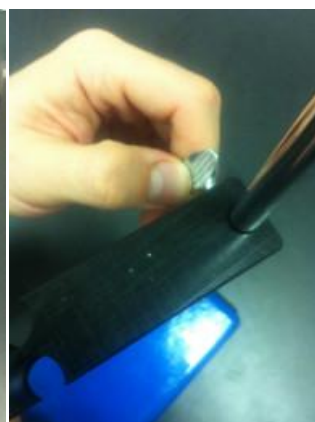
Figure 6. The thumb screw makes adjusting The Vinmetrica Electrode Holder's height easy.
