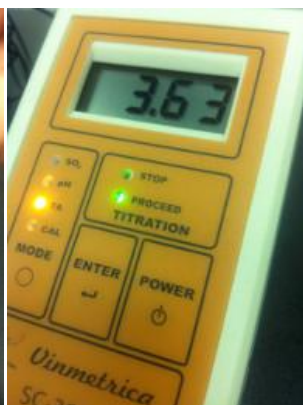
Figure 25. Make sure that the green "PROCEED" LED is lit. You should be reading a pH close to what you expect your wine is at. You are ready to titrate!
