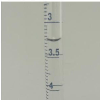
Figure 13. The Meniscus of the water column. This curve is formed because of interactions of water with the glass burette. We recommend measuring the titrant volume from the bottom of the meniscus. In the picture the value is about 3.27 mL.
