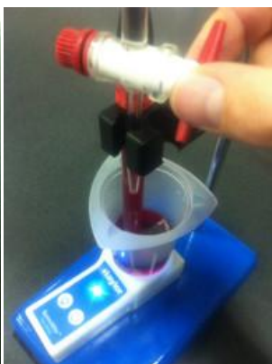
Figure 24. Automated stirring technique. Turn on the magnetic stirrer; add TA Titrant by slowly opening the burette stopcock valve.
