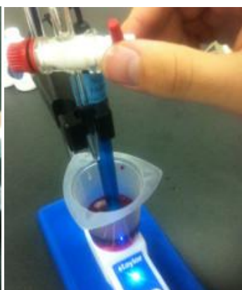
Figure 20. Automated stirring technique. Turn on the magnetic stirrer; add SO 2 Titrant by slowly opening the burette stopcock valve.
