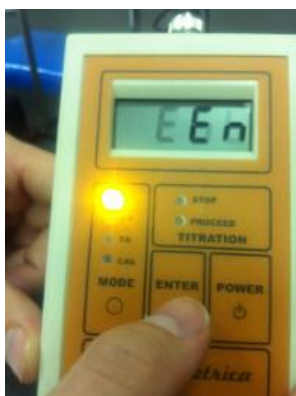
Figure 15. Once in SO 2 MODE the instrument should read 'Press Enter' Press ENTER to activate SO 2 MODE.
