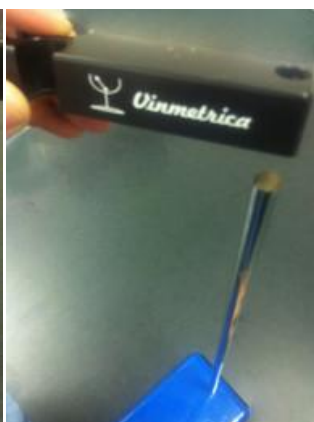
Figure 5. The Vinmetrica Electrode Holder slides onto the Lab Support Stand.
