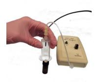
**Figure 7.** Position the opening of the vial insertion assembly over the vial.
