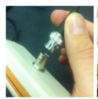
**Figure 2.** Attach the SC-50's cable to the BNC or RCA connector on the SC-300 (or 100)
